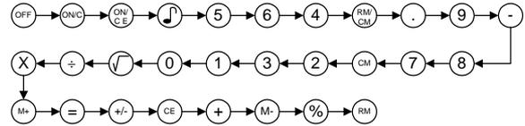
When the OFF and ON/C key are depressed simultaneously, the OFF key is given priority.
